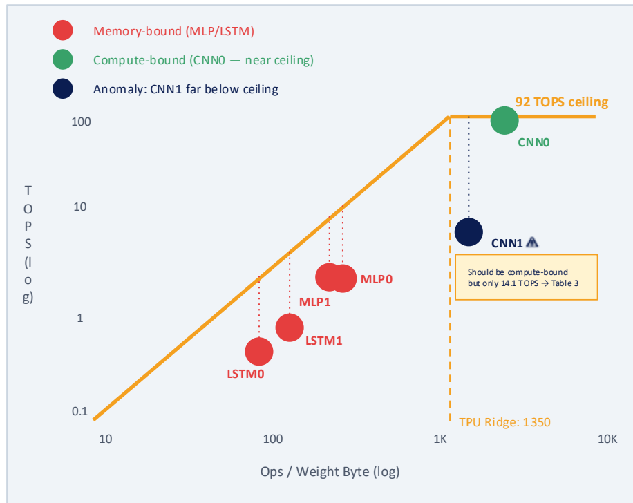
Figure 5 — TPU Roofline: Where the Six Apps Land
